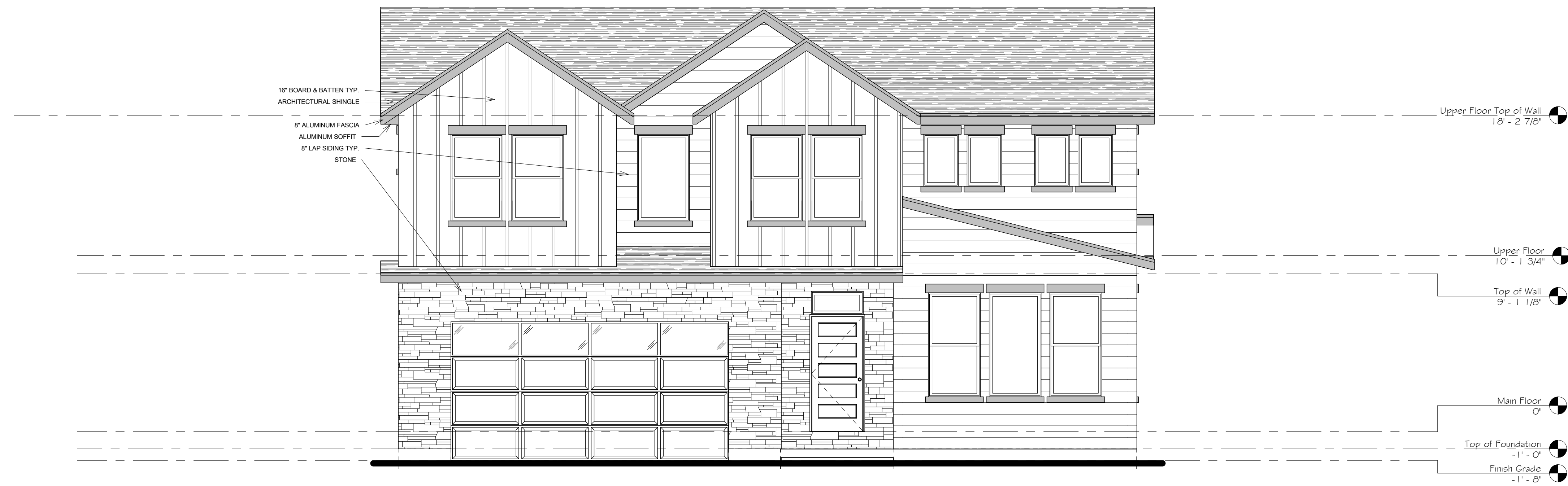
1 Front Elevation (West) A-200 SCALE (24 x 36): 1/4" = 1'-0" SCALE (11 x 17): 1/8" = 1'-0"
